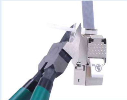
11. Push the cable tie in and lock it. Cut off the excess braided and cable tie
