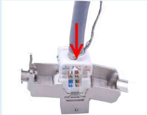
8. Put the cable pressing cover into module line base
