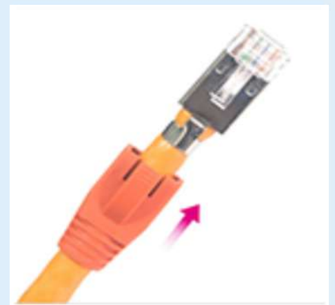
12. Insert the cable cap into the RJ45 plug
