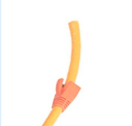
1. Insert the cable cap
