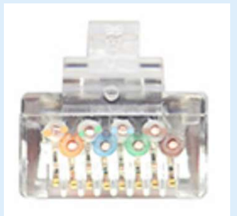
9. Insure that the wires are pushed to the end of the plug's holes
