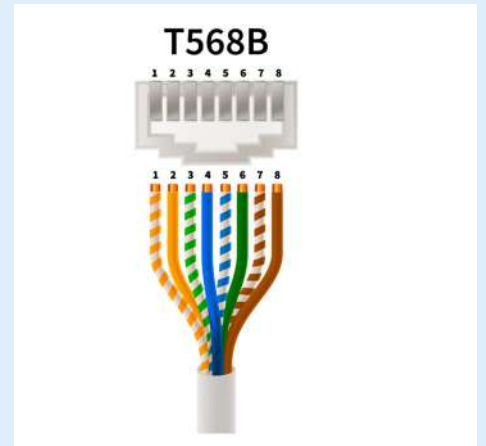
6. Keep the wires neat, T568B
