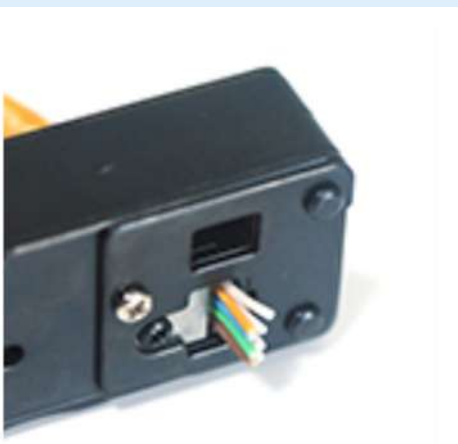
8. Put the plug into the crimping tool. Crimp plug
