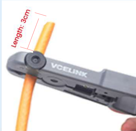
2. Put the Ethernet cable into the stripper
