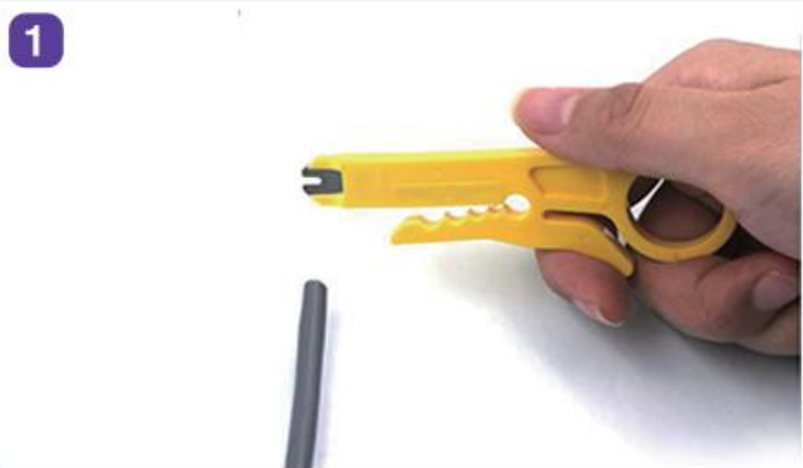
Prepare the mini stripping tool and Ethernet cable.
