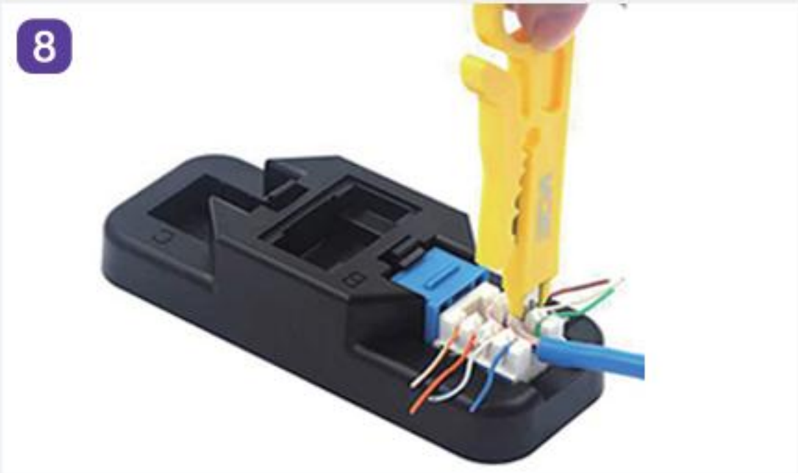
Use the punch down stand mini stripper to punch down the keystone jack.
