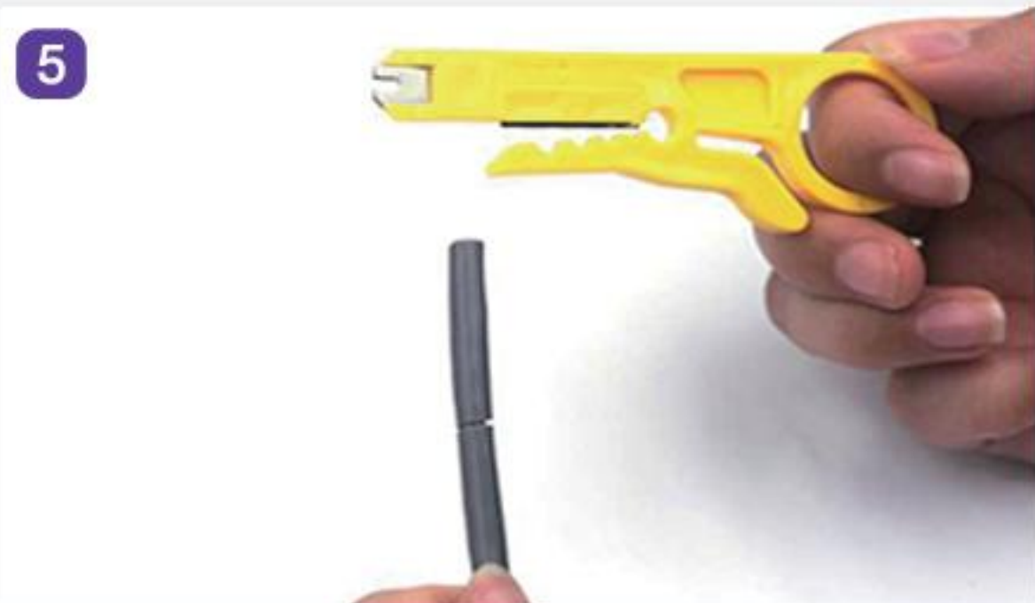
The cable jacket is stripped.
